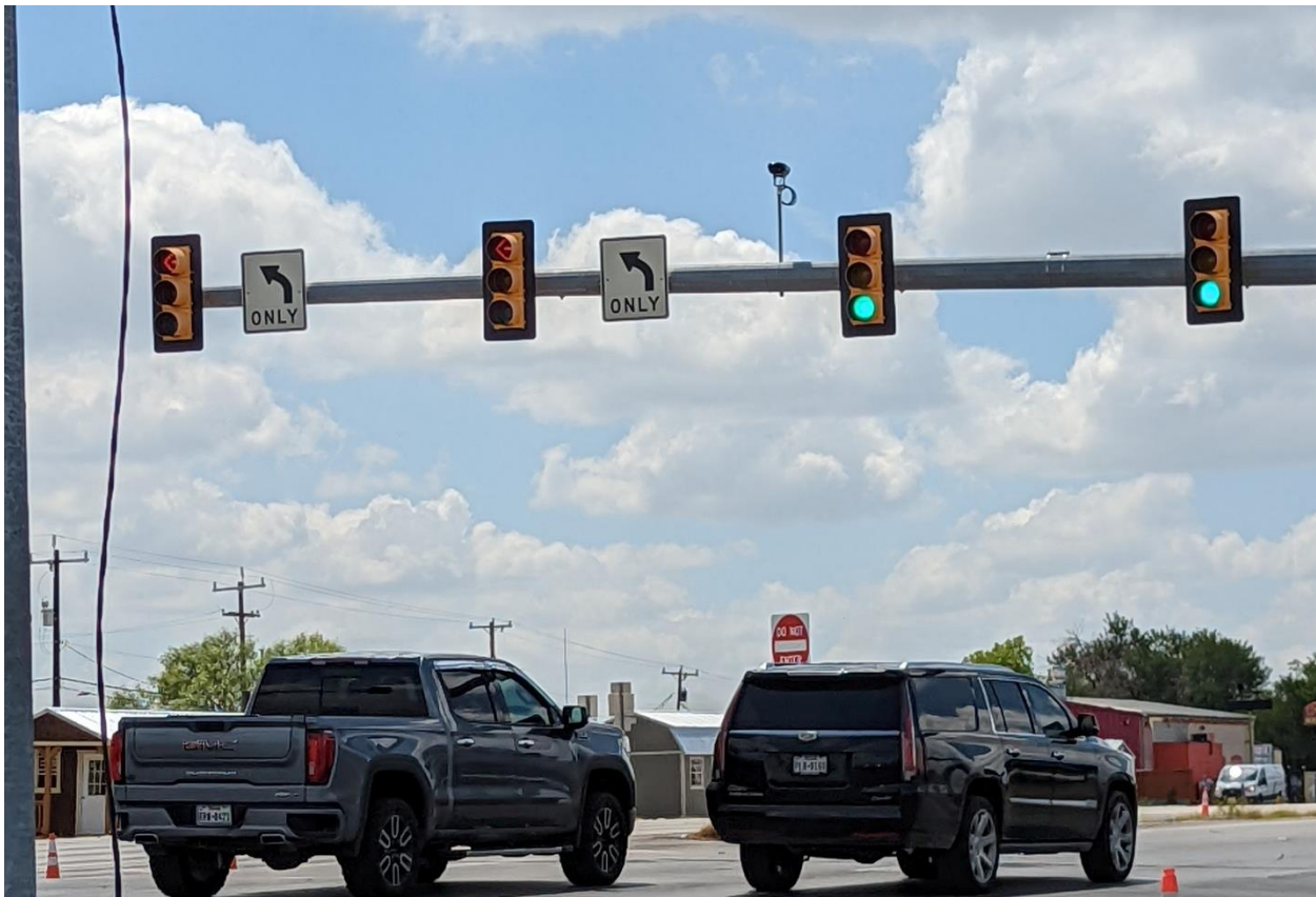
Figure 28: Typical SU mounting - center of the approach at maximum height
