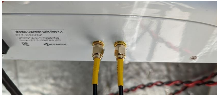
Figure 22: CU Wi-Fi antenna leads
