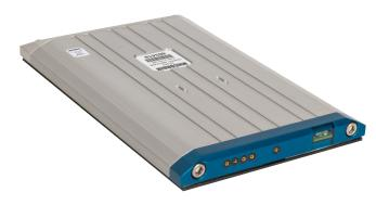
The NC350 BlueStar Portable Traffic Analyzer with Bluetooth™ Technology from MH Corbin provides the accurate measurements of vehicle count, speed, and vehicle length. The NC350 BlueStar Portable Traffic Analyzer sensor is placed directly in the traffic lane to measure data, and can be installed and removed quickly and easily without damage to the road surface.
