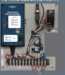
\*Upgrade an outdated TAPCO system or a non-TAPCO system with the BlinkLink enabled 4G Time Clock Retrofit Kit
