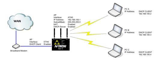
The 702-W configured as a powered router allows Layer 3 routing to setup network segmentation. It supports the Network Address Translation (Masquerading) feature which is widely used by access points. NAT will act as the firewall between LAN and WLAN networks. Additional firewall settings can be configured for Layer 3 packet filtering and access control in router mode. It can also act as a DHCP server, automating the assigning of IP addresses.
