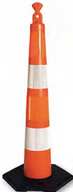
42" Grabber-Cone with (2) 6" orange and (2) 6" white bands of 3M™ diamond grade reflective sheeting
