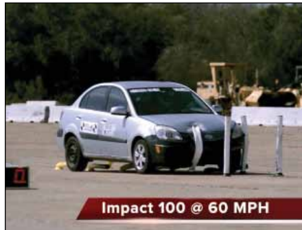
City Posts rebound to vertical, even after 100 hits at 60 mph
