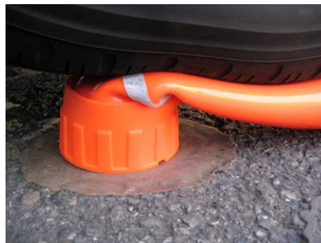
City Posts withstand low-speed crushing forces
