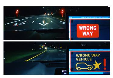
3 In-vehicle alerts provide wrong-way and rightway drivers with instant notifications through connected vehicle dashboards, rear view mirrors and mobile devices.
